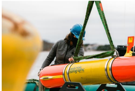
Figure 41: a two pick, lighter lifting bail system was developed for the helicopter demonstration.
