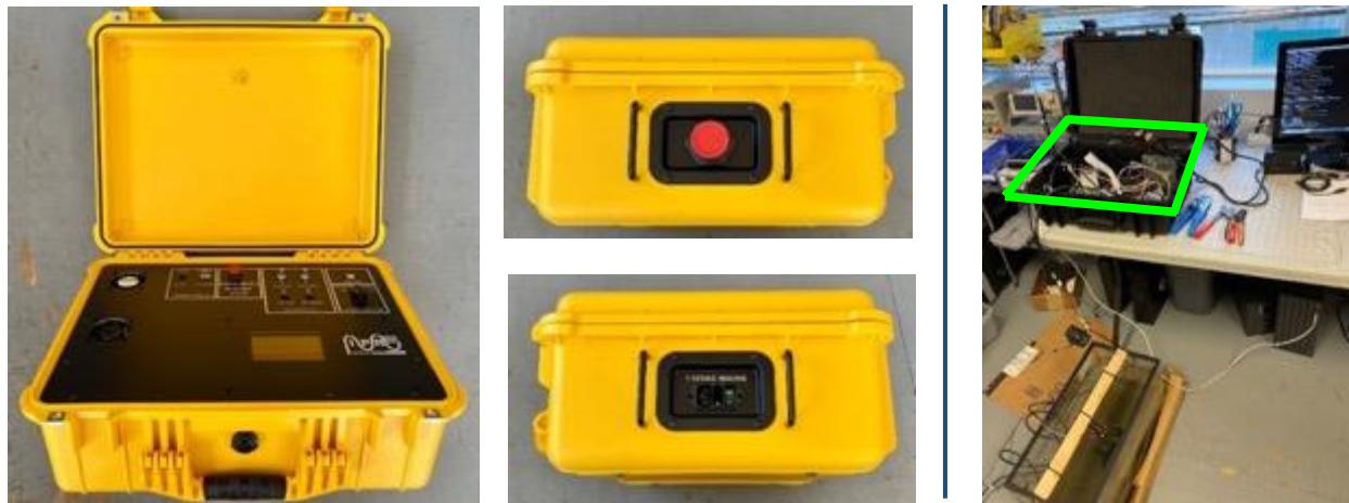
(Left and Center) Customized Marine IP system enclosure showing cooling fans, operating switches, and a touch screen. (Right) The laboratory testing apparatus for testing components and laboratory system performance.
